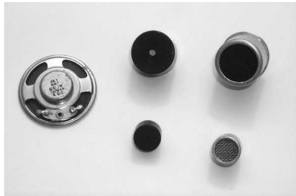
Figure 15.3 A selection of audible transducers
