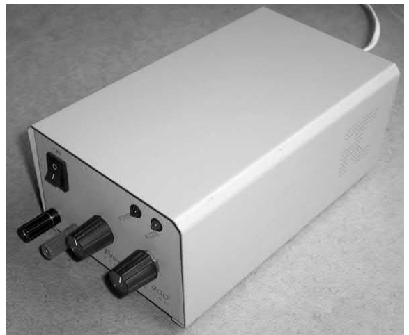
Figure 20.50 External view of the bench power supply showing the front panel controls and enclosure
