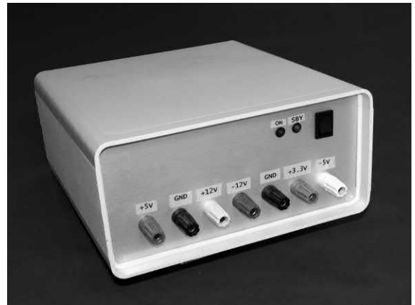
Figure A10.3 The author's ATX-based power unit makes a handy bench supply
