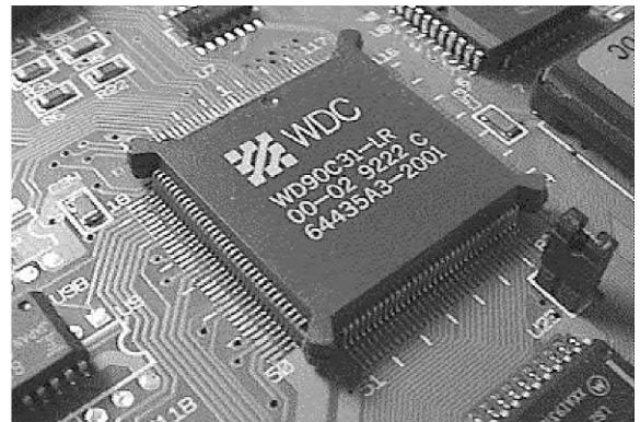
Figure 5.37 A large-scale integrated (LSI) circuit mounted in a socket fitted to a printed circuit board
