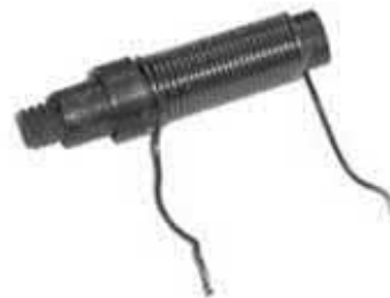
Figure 2.43 An adjustable ferrite-cored inductor
