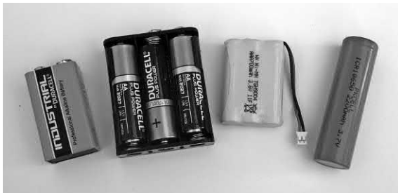
Figure 6.32 Some typical battery packs for small electronic equipment. From left to right: alkaline a 9 V PP3 based on six layered 1.5 V cells; a 4.5 V battery pack based on three 1.5 V alkaline cells; a 3.6 V pack based on three Ni-MH cells; a single 3.7 V high-capacity Li-ion cell.
