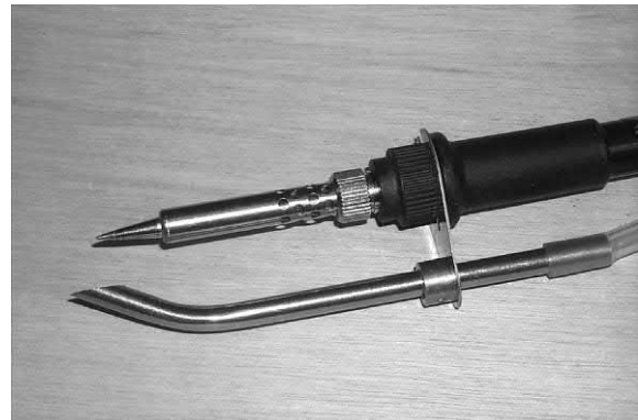
Figure 20.17 Fume extraction facility which can be added to a temperature-controlled iron when necessary
