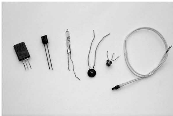
Figure 15.6 Various temperature and gas sensors
