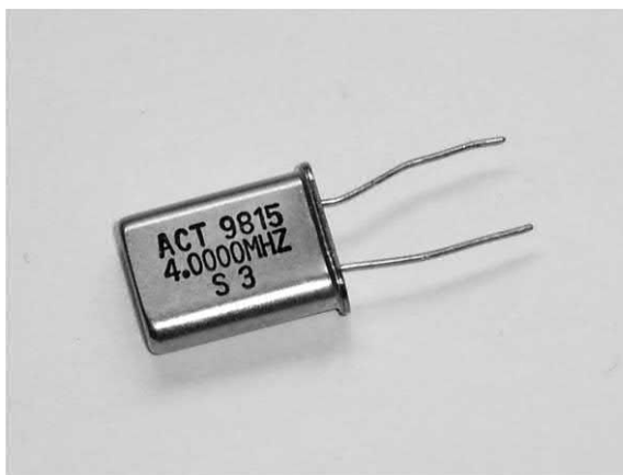
Figure 9.11 A quartz crystal (this crystal is cut to be resonant at 4 MHz and is supplied in an HC18 wire-ended package)
