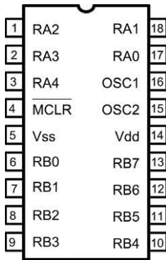
Figure 17.2 Pin connections for the PIC16C84 and PIC16F84 devices
