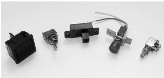
Figure 1.20 Various types of switch. From left to right: a mains rocker switch, an SPDT miniature toggle (changeover) switch, a DPDT slide switch, an SPDT push-button (wired for use as an SPST push-button), a miniature PCB mounting DPDT push-button (with a latching action)
