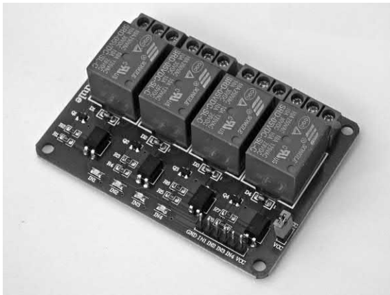
Figure 19.24 A four-channel relay interface
