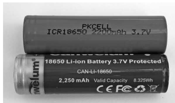
Figure 6.35 Protected (bottom) and unprotected (top) 3.7V 18650 cells
