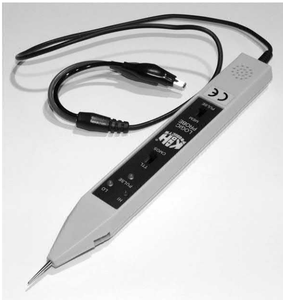
Figure 14.17 A versatile logic probe with logic level and pulse indicating facilities. Note the crocodile leads for connecting to the TTL or CMOS supply and ground connections
