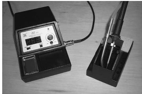
Figure 20.16 A modern temperature-controlled soldering station with ESD and fume extraction facilities
