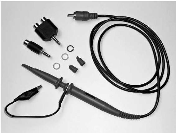
Figure 13.42 The Virtins (see Appendix 9) sound card oscilloscope probes are designed to be connected directly to the audio input jack connectors of a PC
